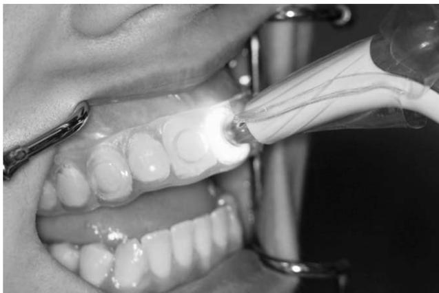
Figure 1. Positioner for the digital spectrophotometer.
